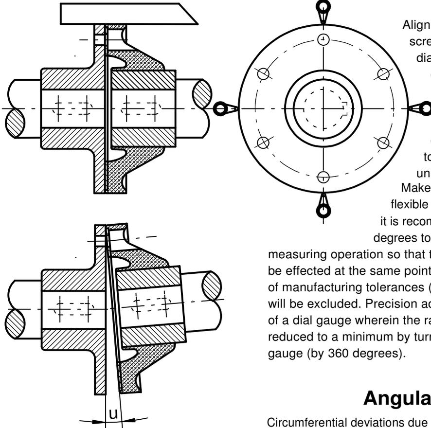
Align the Kegelflex-Coupling without head screws inserted. Using a straightedge (or a dial gauge in case of higher speeds), determine the radial runout of coupling discs in relation to each other at 4 measuring points offset by 90 degrees (if access is difficult 3 points at 120 degrees will be sufficient) and reduce it to a minimum by alignment of the machine units connected.
